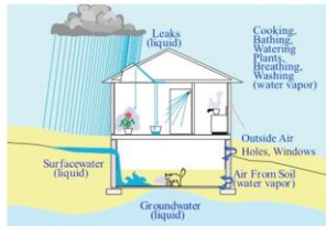
Figure 4.11 Ways in Which Water Can Enter a Building (Envelope leaks can occur from anywhere in the building roof, windows, walls, doors and penetrations)
